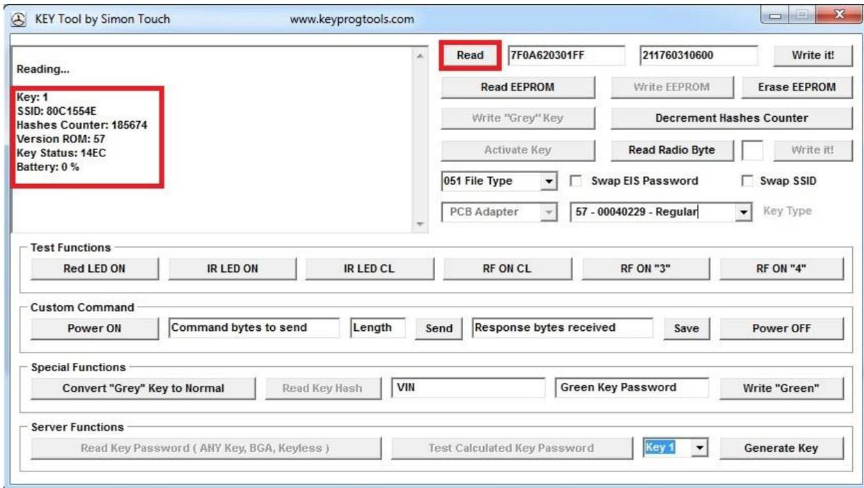
12 – Click on READ EEPROM, device will take 10 to 20 seconds to read the password and it will automatically save the password in Read folder.
