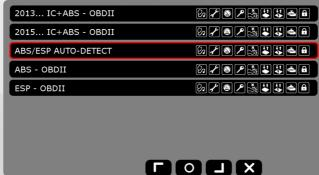
After using AUTO-DETECT function DiagProg4 will indicate program number needed to correct odometer or if it is already active required program will be launched.
